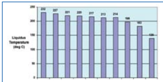
Figure 1. Liquidus Temperature of some lead-free solders compared with that of Sn-37Pb.
