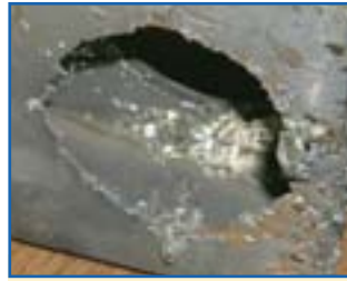
Figure 2. Erosion of stainless steel wave solder pump sump by SnAgCu lead-free solder.
